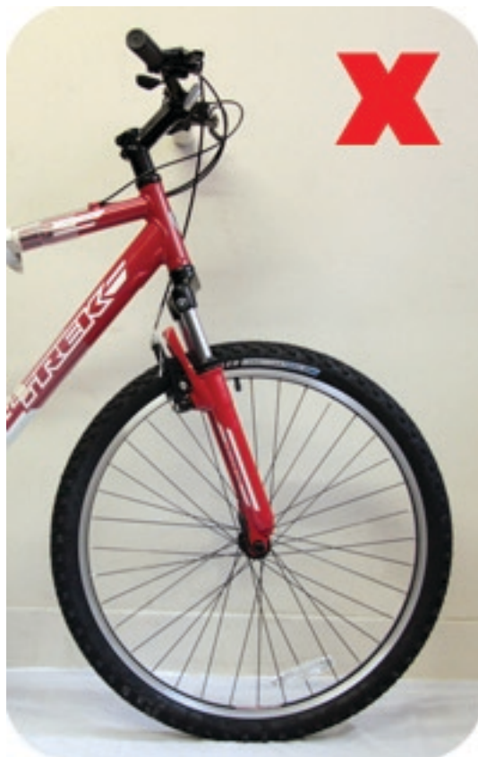
2. Position the fork so rim brake is at the front.
