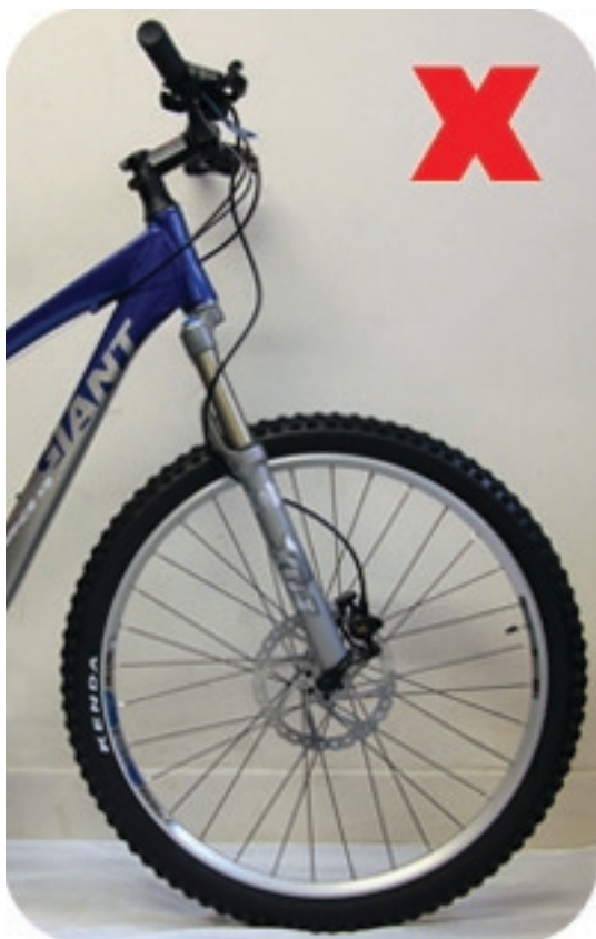
1. Position the fork so disc brake caliper is at the rear.
