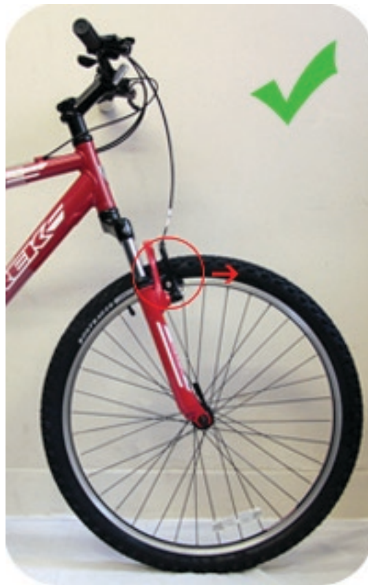
2. Position the fork so rim brake is at the front.
