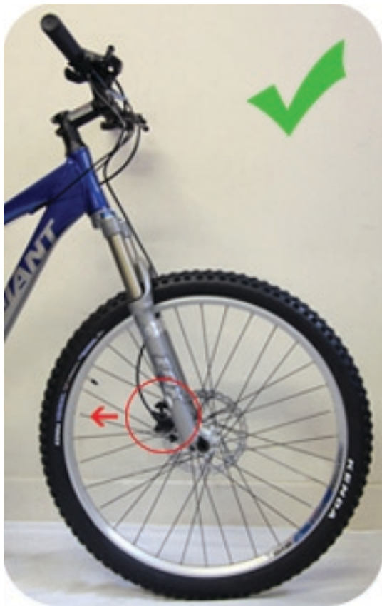
1. Position the fork so disc brake caliper is at the rear.
